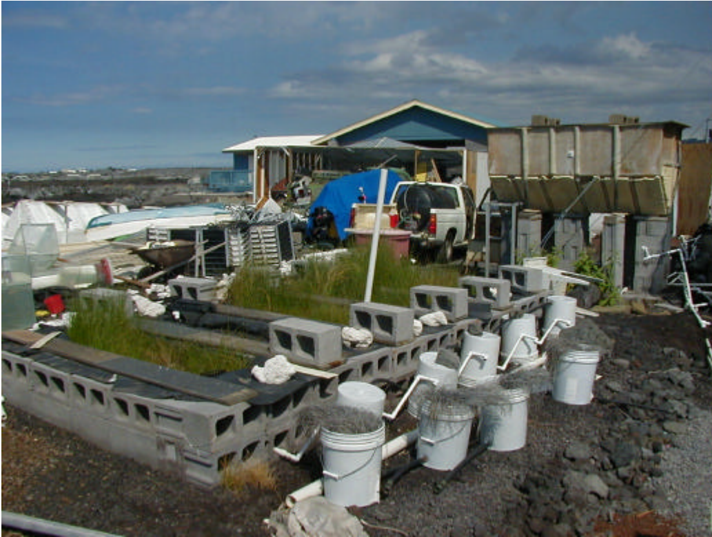
Fig. 2. The experimental set up at WHEA. In the background is the elevated holding tank for system influent. Five cells (one unvegetated) are visible in the foreground
